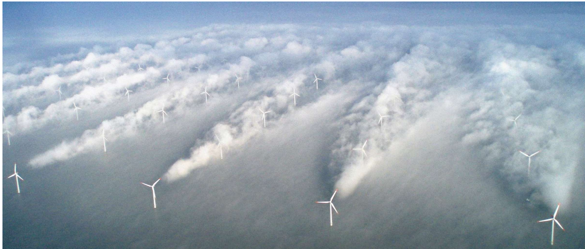
Figure 1: example of a wake effect at Horns Rev wind farm off the Danish coast where turbines mix humid air to higher colder levels where the air condensates and forms clouds (source: Vattenfall).
